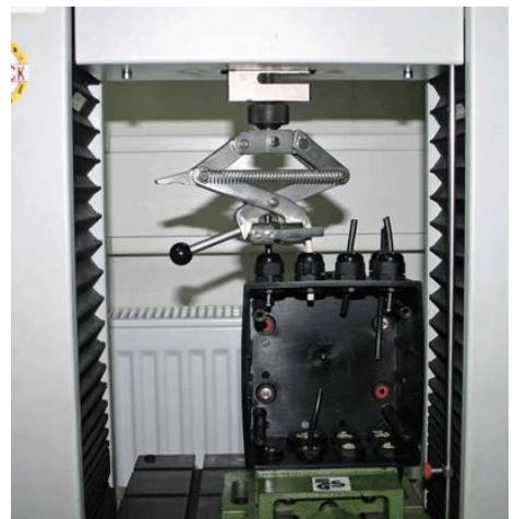
Cable extraction force - junction box
